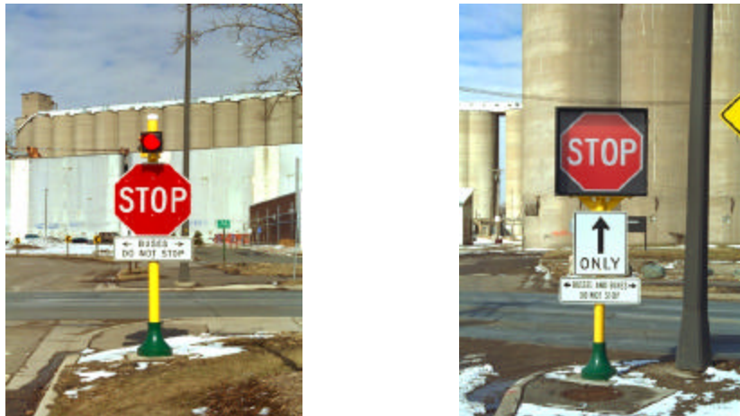
Figure 4. Loop detector activated warning & stop signs
